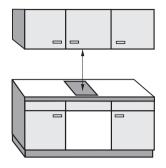
A minimum safety distance must be maintained between the appliance and the cooker hood above it. See the cooker hood manufacturer's operating and installation instructions for details.
